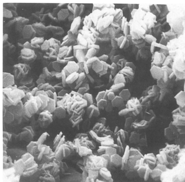
Figure 2 Scanning electron micrograph of the Mg(OH) 2 used with particles in the form of hexagonal plates (Kyowa, Japan). \times 3922 .
